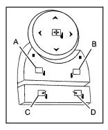
The power mirror controls are located on the driver's door armrest and operate both outside rearview mirrors.
